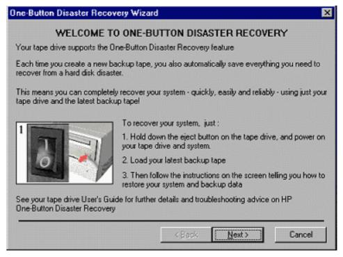
Once the HP OBDR drive has been identified, the installation utility informs the user. This is an opportunity to explain what steps are necessary to test the HP OBDR functionality and make the first, real backup that is protected by HP OBDR.
