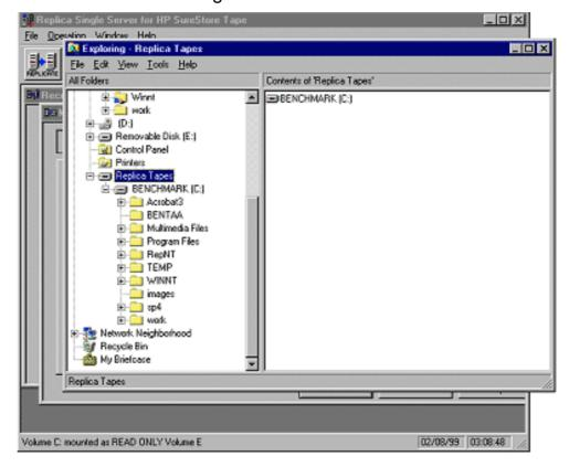
Obviously, this functionality is specific to the backup software package, in this case Replica Single Server for HP SureStore Tape, but it illustrates well the transparency of the HP OBDR system. If a basic tape drive had been used instead of one with HP OBDR capability, the backup cartridge would have been mounted and accessible in exactly the same way.
