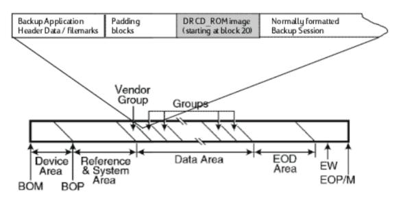
Once switched into HP OBDR mode, the DDS tape drive waits and checks any cartridge it receives for a disaster recovery header. Any non-DR cartridge is ejected, but once it detects a DR cartridge, it proceeds to read the special DR CD-ROM image block, and the computer boots from this code.
