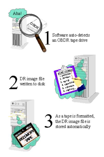
At this point the backup cartridge is theoretically just about usable for disaster recovery (although the full system could not be restored without an earlier backup). The backup cartridge becomes fully DR-capable once the first normal backup completes. Until then, it does not contain all the data files.
