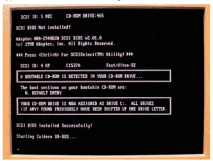
This screen indicates that the tape drive has been detected as a bootable CD-ROM. The line immediately above the "A Bootable CD-ROM&" message shows that the tape drive is attached to the SCSI adapter at ID 4.
