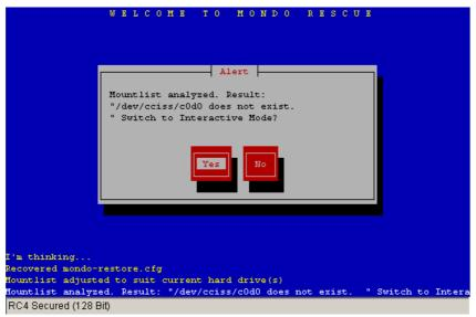
Edit the mountlist and change the devices to reflect the current hardware (going from /dev/c0d0 to /dev/sda or /dev/sdb for the SATA controller). In this example, the source disks were 36Gb and the target ones were 80Gb.
