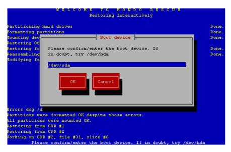
Then it will ask to review the /etc/fstab, /etc/grub.conf files before rebooting the server. For fstab, you should change the file to reflect the change of hard drive reference (in our case from /dev/cciss/c0d0p? To /dev/sda?) as in the lines below. If you are using Label on drives, you can stay with it, Mondo will handle it properly.
